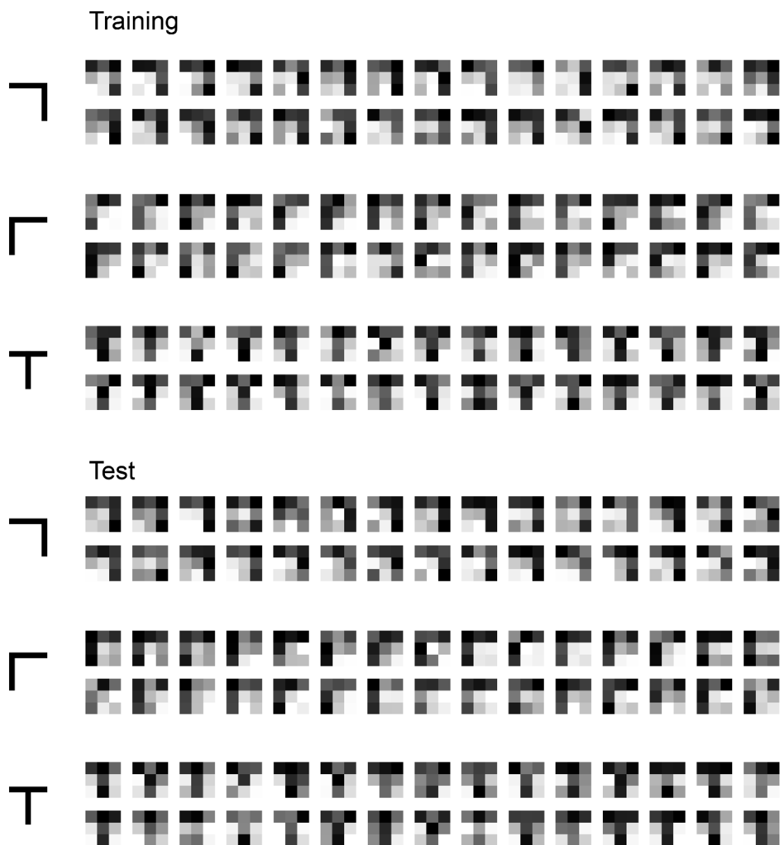
Fig. S52 Custom symbolic dataset used for classification and autoencoding tasks. Example images from the training and test sets of a custom 3 \times 3 -pixel symbolic dataset. The dataset includes three classes ('┐', '┌', and '└'), each corrupted with randomly generated noise to simulate real-world distortions. A total of 600 images were used for training and 150 for testing. This dataset was employed to evaluate the performance of the Fe-FET-based system on both supervised classification and unsupervised reconstruction tasks.
