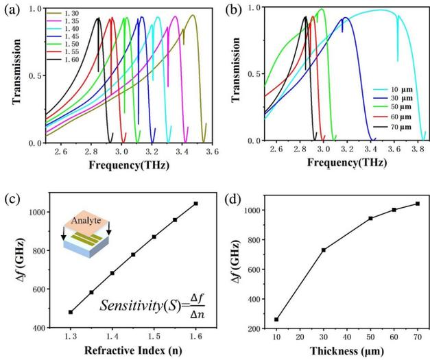
**Fig. 7.** (a) Dependence of transmission on the refractive index increased from 1.3 to 1.6 under the thickness of 70  $\mu\text{m}$ ; (b) dependence of transmission on the analyte thickness increased from 10 to 70  $\mu\text{m}$  under the refractive index of 1.6; (c) frequency shift under different refractive indices of analyte extracted from [a]; (d) frequency shift under different analyte thicknesses extracted from [b].
