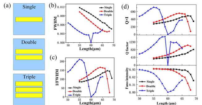
**Fig. 4.** (a) Single, double, and triple metal bars structure unit; (b) FWHM under different lengths; (c) ratio of Fano intensity to FWHM under different lengths; (d) Fano intensity,  $Q$  factor, and  $Q \times I$  under different lengths.
