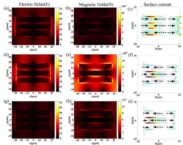
**Fig. 6.** (a), (d), (g) Electric, (b), (e), (h) magnetic fields, and (c), (f), (i) surface current at the Fano resonance. (a), (b), (c) The length is 59  $\mu\text{m}$ ; (d), (e), (f) the length is 55  $\mu\text{m}$ ; (g), (h), (i) the length is 50  $\mu\text{m}$ .
