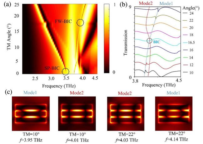
**Fig. 8.** Angular response for the triple metal bar length of 55  $\mu\text{m}$ : (a) simulated transmission contour plot under TM-polarized incidence; (b) simulated transmission curves with incidence angles from 10° to 24°; (c) field distribution of Mode 1 and Mode 2 at 10° and 24°, respectively.
