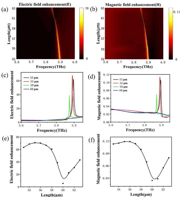
**Fig. 5.** Simulated field enhancement of the triple metal bars. (a) and (b) show color plots of the field enhancement for different lengths in the triple metal bars, respectively; (c) electric field enhancement and (d) magnetic field enhancement for the lengths of 53, 55, 59, and 60  $\mu\text{m}$  in the triple metal bars, respectively; (e) electric field enhancement and (f) magnetic field enhancement corresponding to the green dotted lines in (a) and (b), respectively.
