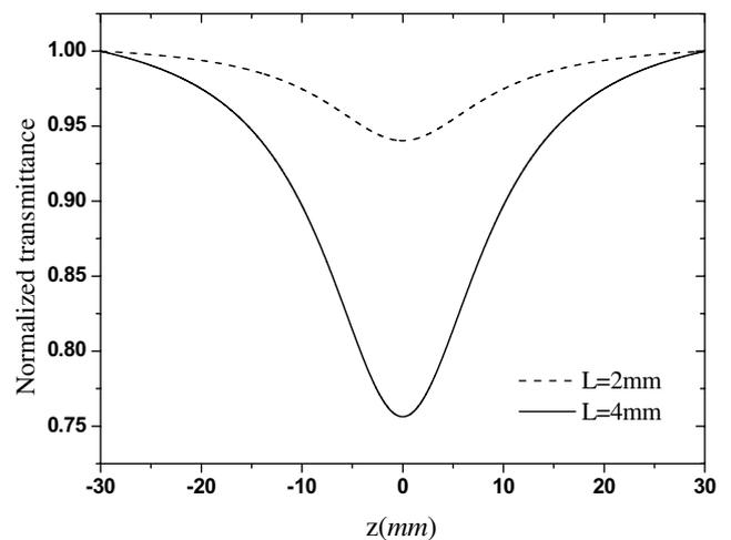
Fig. 1. The Z-scan curves for different  $L$ .
