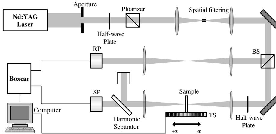
Fig. 5. The Z-scan experimental setup. BS, beam splitter; SP, signal probe; and RP, reference probe.
