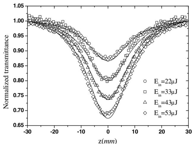
Fig. 6. The experimental and theoretical Z-scan curves of 5%MgO:LiNbO<sub>3</sub> crystal for different incident energy  $E_{\text{in}}$ . The solid lines represent the theoretical fittings, where  $\alpha_{\omega} = 0.03 \text{ m}^{-1}$ ,  $\alpha_{2\omega} = 2 \text{ m}^{-1}$ , and  $\Delta kL = 3.8$ .
