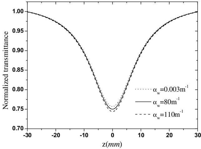
Fig. 2. The Z-scan curves for different linear absorption coefficients of fundamental light, where  $E_{in} = 40 \mu\text{J}$ ,  $\omega_0 = 38 \mu\text{m}$ ,  $L = 4 \text{ mm}$ , and  $\Delta kL = 3.8$ .
