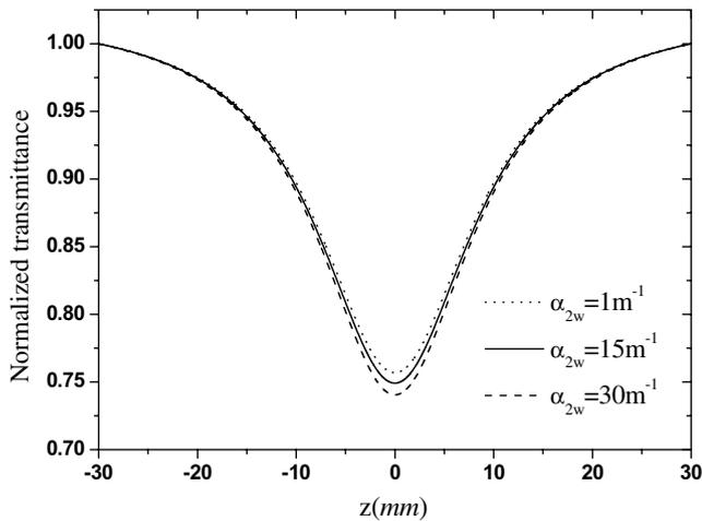
Fig. 3. The Z-scan curves for different linear absorption coefficients of SH light, where  $E_{in} = 40 \mu\text{J}$ ,  $\omega_0 = 38 \mu\text{m}$ ,  $L = 4 \text{ mm}$ , and  $\Delta kL = 3.8$ .
