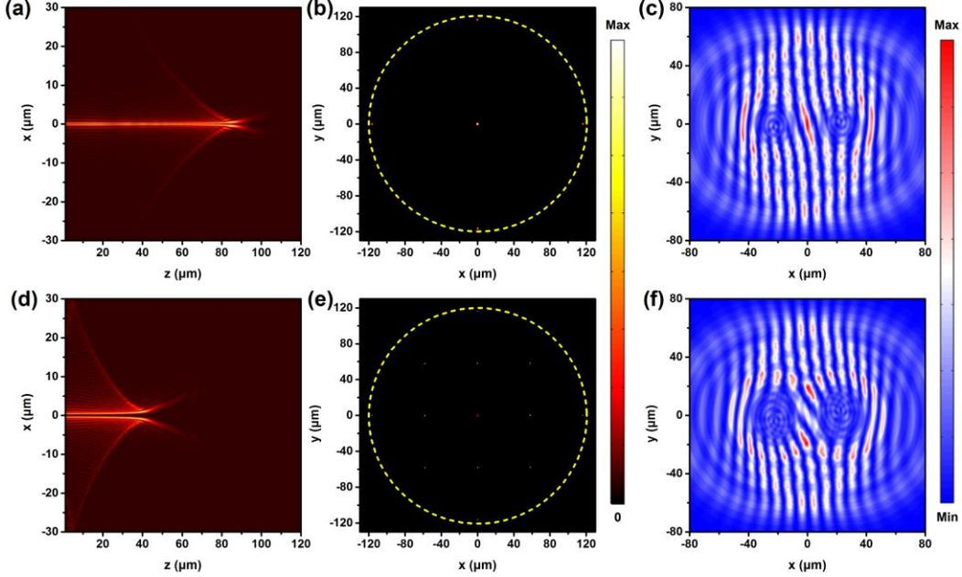
**Figure S4.** Numerical intensity profile (a), intensity distribution at focal plane (b) and self-interference pattern after the phase mask plane (c) of the THG optical vortex with spin  $\sigma$ . Numerical intensity profile (d), intensity distribution at focal plane (e) and self-interference pattern after the phase mask plane (f) of the THG optical vortex with spin  $-\sigma$ .
