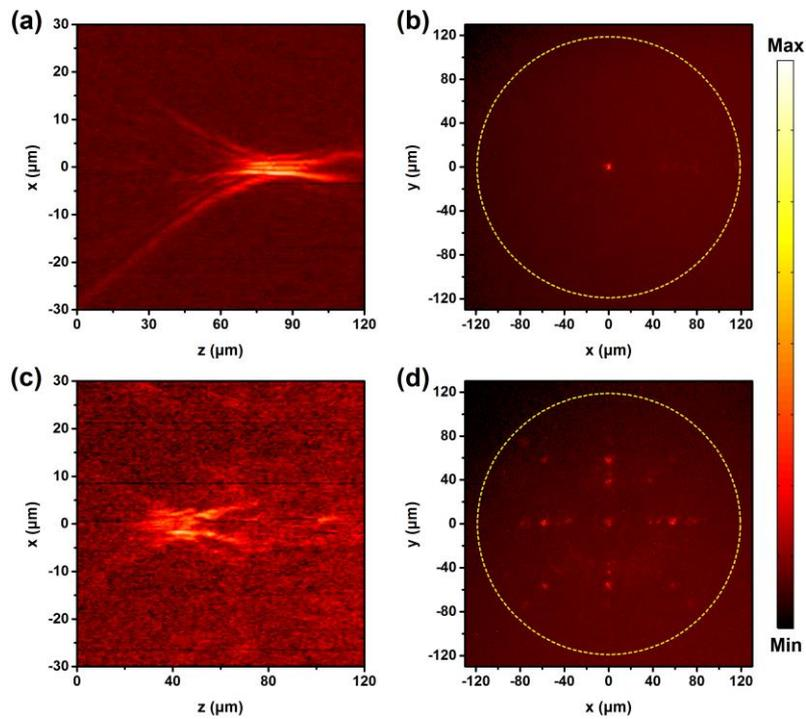
**Figure S3.** Measured intensity profile along the propagation direction (a) and intensity distribution at focal plane (b) of the THG optical vortex with spin  $\sigma$ . Measured intensity profile along the propagation direction (c) and intensity distribution at focal plane (d) of the THG optical vortex with spin  $-\sigma$ . The scale bar is adapted for each figure.
