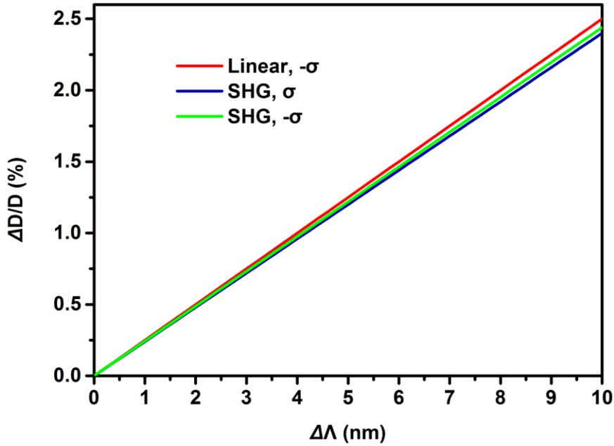
**Figure S1.** Calculated disturbances  $\Delta D/D$  of the linear and SHG optical vortices as functions of tolerance in the period of meta-atom  $\Delta\Lambda$ .
