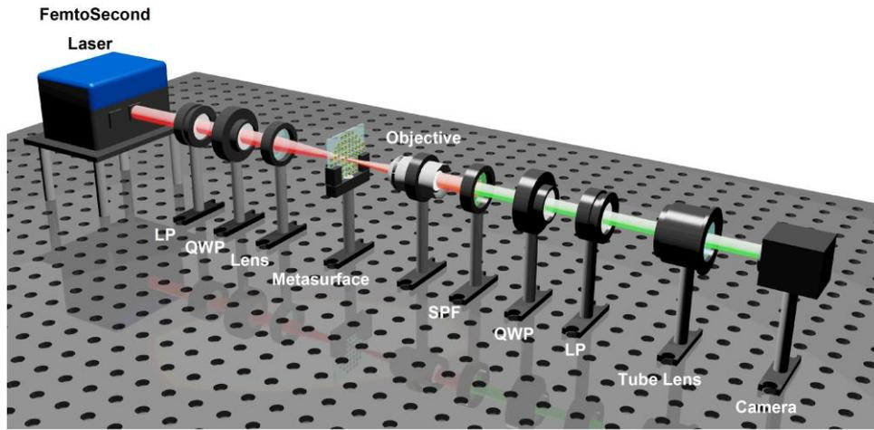
**Figure S1.** Illustration of the measurement set-up for measuring focal lengths and capturing optical vortices.
